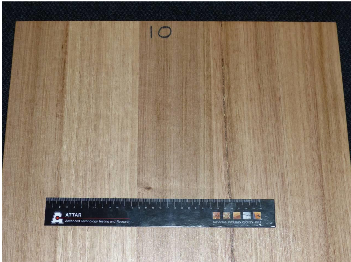
Figure 1: One coat FASTASEAL 3030 Clear Sealer. One coat POLYTHANE 2043 A&B Two Pack. One coat POLYTHANE 2043 A&B Two Pack containing Polycure 3920 High Grip applied to timber board.
